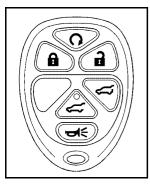
Press to unlock the driver door. Press again within three seconds to unlock all remaining doors. Press **f** to lock all doors.
